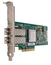
2500 Series. The 2500 Series adapters are designed to meet the business requirements of the enterprise data center by enabling the lowest possible power consumption and the highest level of data protection. These adapters interface to the host server with a PCle® Gen2 bus, ensuring no internal performance bottlenecks.
