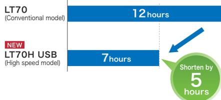
LT70H USB achieves a 70% improvement in data transfer speed over the conventional LT70 USB. It can be used easily on laptop PCs that can not install SAS interface. Because data transfer speed has drastically improved to 240MB/s, it realizes a stress-free backup/archive.
